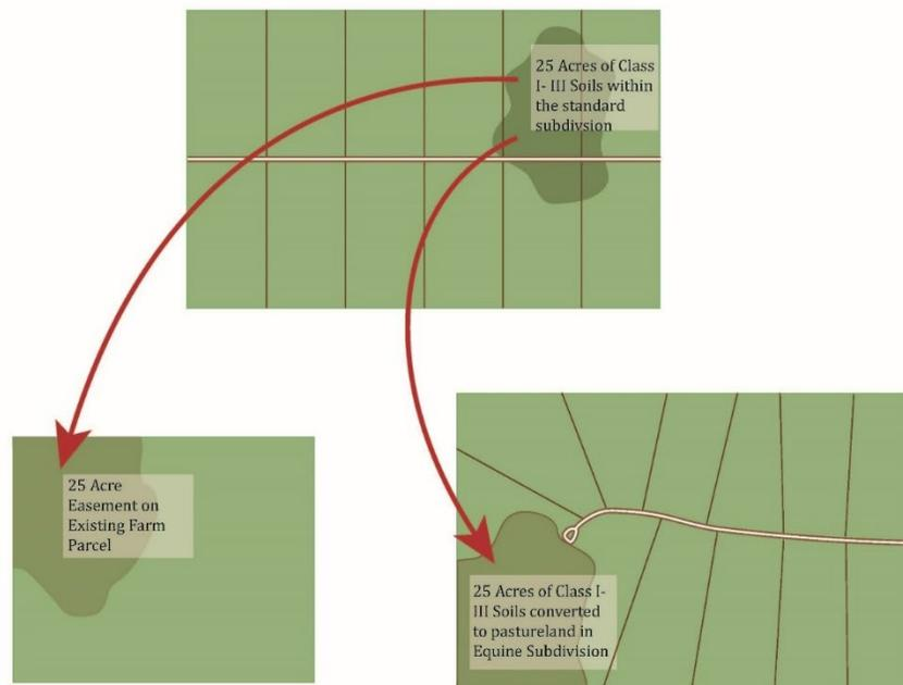
Figure 1: Soil mitigation technique
